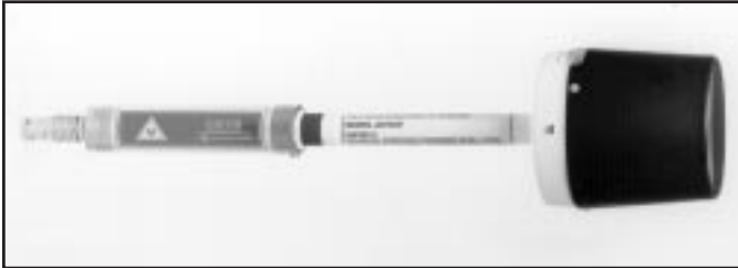
Photo 1. A shaped probe is physically identical to a standard isotropic probe. The difference between the two lies in the shaped probe's frequency response curve, which is "shaped" to mimic the requirements of a major standard.
